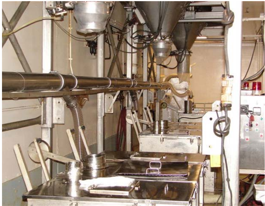
Three dumping stations where the powdered soup ingredients are mixed.
