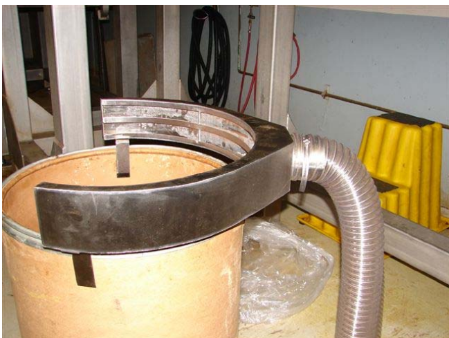
Horseshoe Hoods for capturing fugitive dust when powdered ingredients are dumped into drums.
